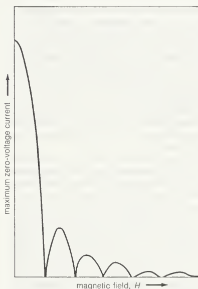
Figure 51: Maximum zero-voltage (Josephson) current passing through a junction by Cooper-pair tunneling as a function of magnetic field.
